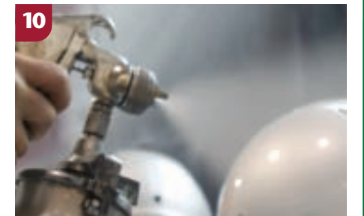
10 Spray booths provide painters with a moving line of primed helmets. As helmets approach the booth, they spin to facilitate the smoothest application of paint.
